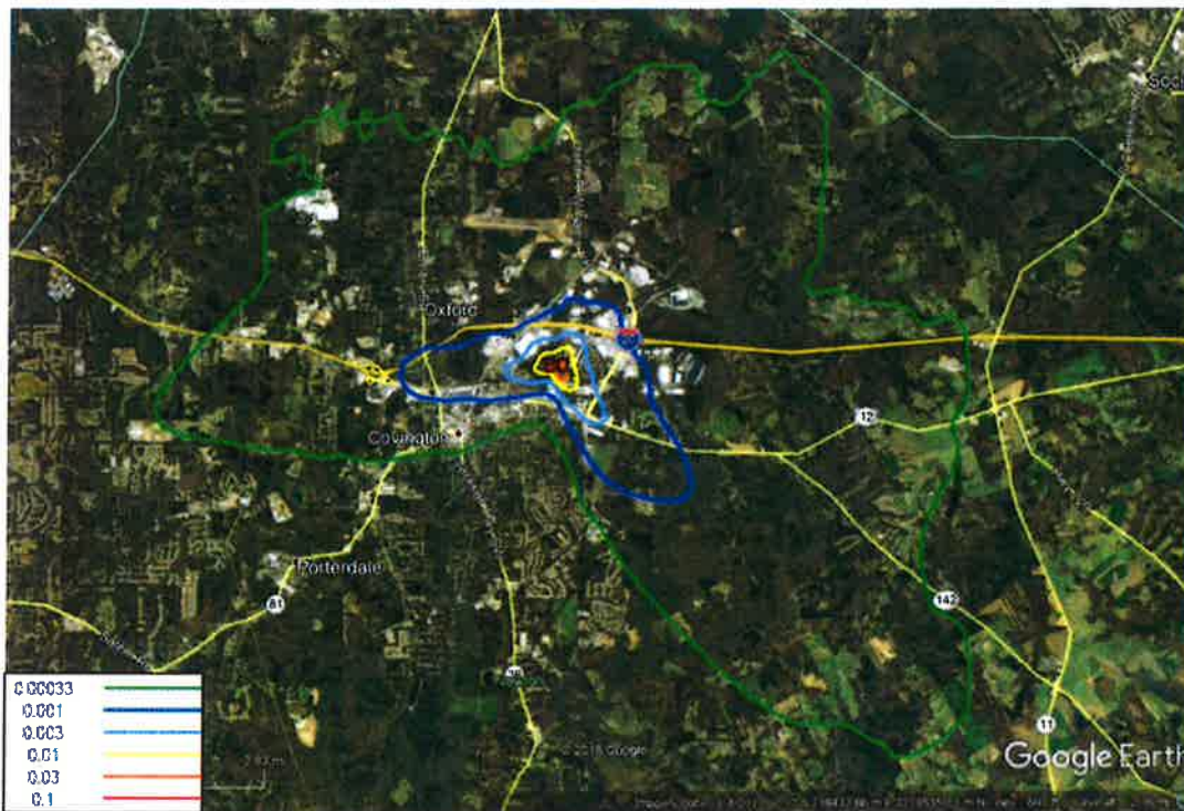
Figure 3. Contours of 5-year annual average ground-level concentrations modeled overlaid on a Google Earth map.
